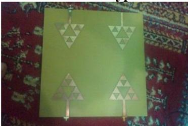
Gambar 4 Gambar Prototype Antena MIMO
