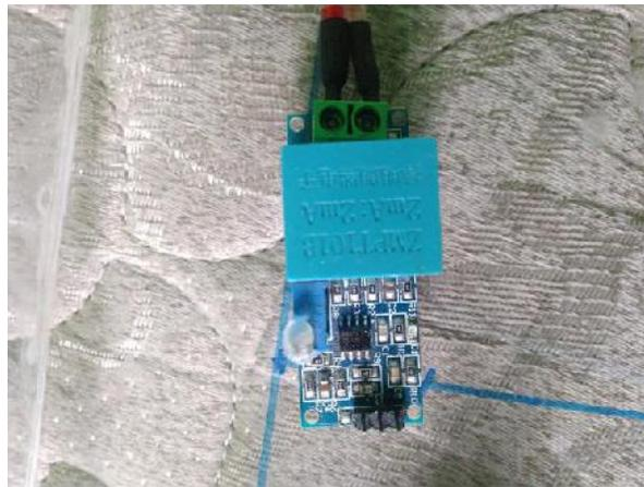
**Gambar 2.2 Sensor tegangan ZMPT101B**
