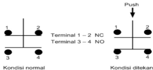
Gambar 2.8 Prinsip Kerja Push Buttom Sumber: http://trikueni-desain-sistem.blogspot.com
