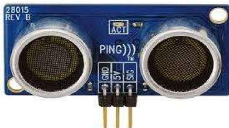
**Gambar 2.3 Sensor Ultrasonik Ping**
