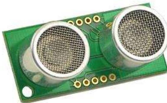
**Gambar 2.2 Sensor Ultrasonik SRF05**
