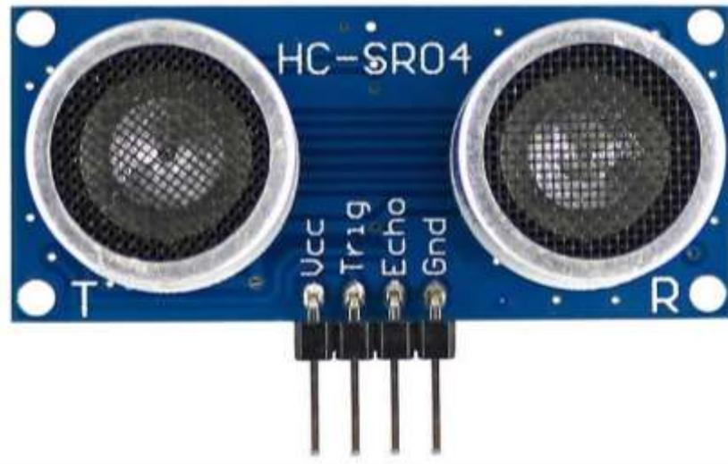
**Gambar 2.1 Sensor Ultrasonik HC-SR04**
