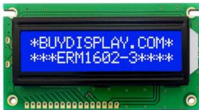
**Gambar 2.8 LCD 2x16**
