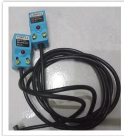
**Gambar 2.5 Sensor Proximity Induktif**
