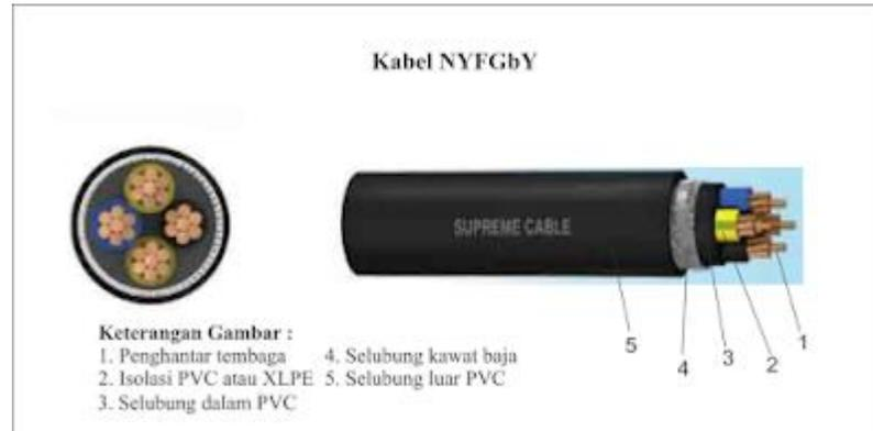
Gambar 2. 8 Kabel NYFGbY (Sumber : <https://www.blogteknisi.com/2016/05/mengenal-9-jenis-kabel-listrik.html>)
