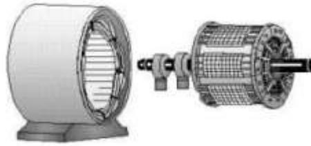
**Gambar 2.12 Motor AC Sinkron**
