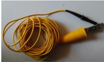
**Gambar 2. 20 Kabel Kuning Earth Tester**
