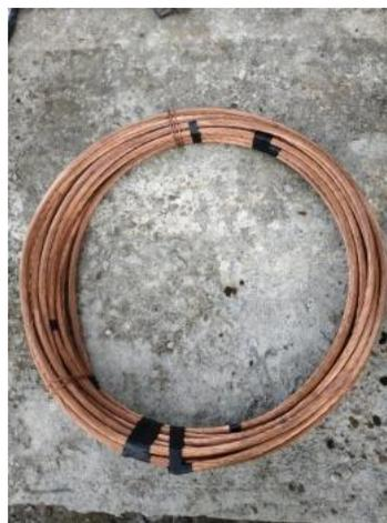
**Gambar 2. 10 Kabel Grounding**
