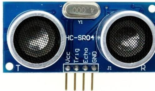
**Gambar 2.5 Sensor Ultrasonik**
