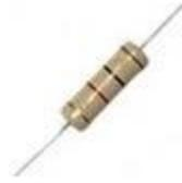
**Gambar 2.14 Resistor Film Karbon**
