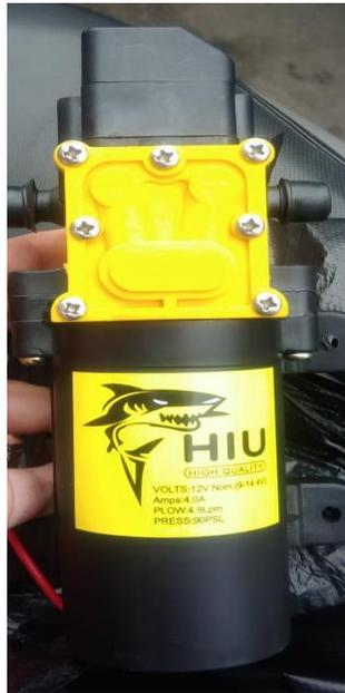
**Gambar 2.9 Pompa Air**
