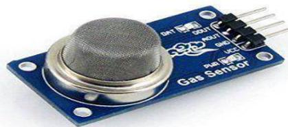
**Gambar 2.4 .** Sensor Asap Mq2
