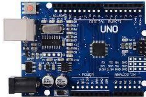
**Gambar 2.2** Board Arduino
