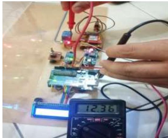
**Gambar 4.10 Tegangan Output Relay Ke Pompa Air Saat ON**
