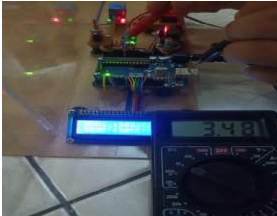
**Gambar 4.5 Tegangan *Output* Sensor Kelembaban Tanah “50%”**
