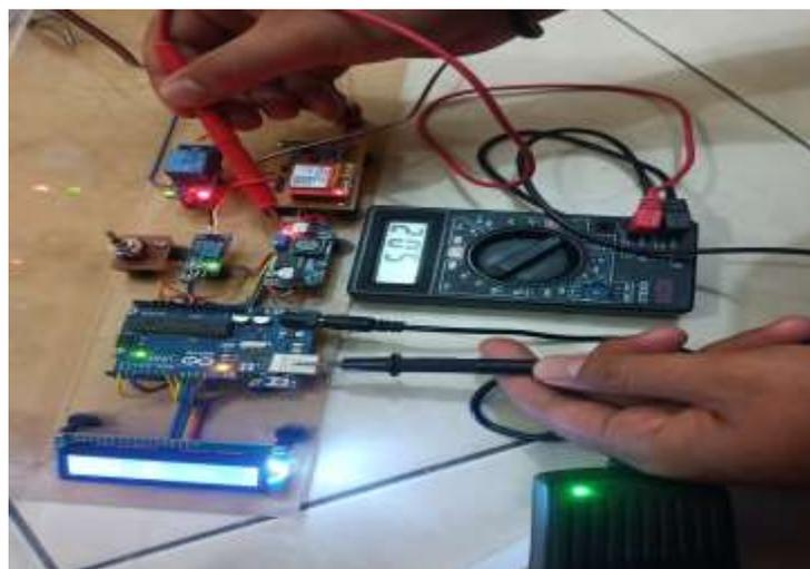
**Gambar 4.2 Pengujian Tegangan *Output LM2596***
