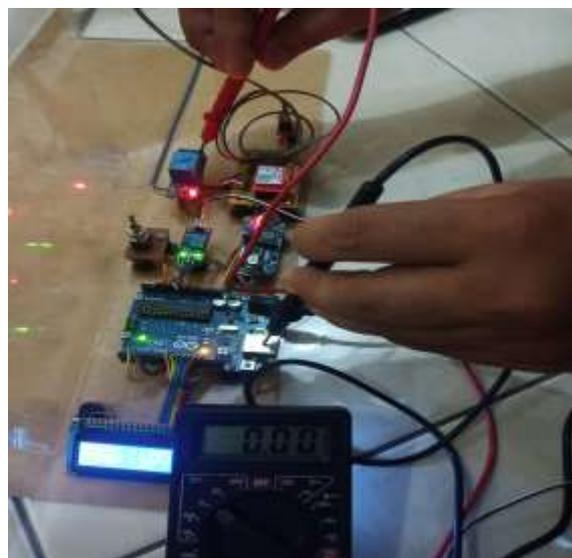
**Gambar 4.11 Tegangan Output Relay Ke Pompa Air Saat OFF**
