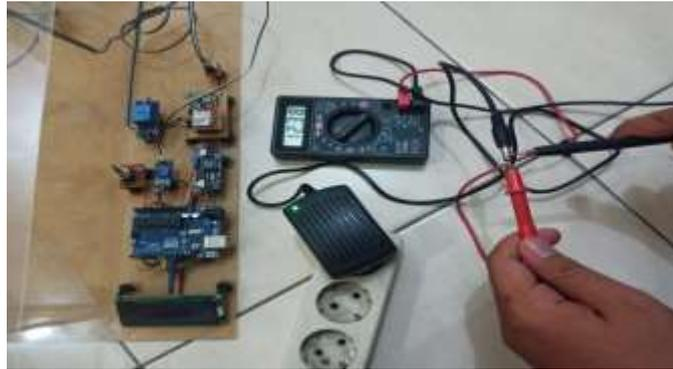
**Gambar 4.1 Pengujian Tegangan Output Power Supply**
