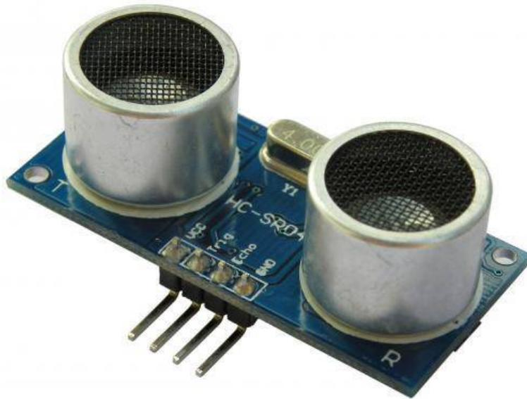
**Gambar 2.1** Sensor Ultrasonic HC-SR04
