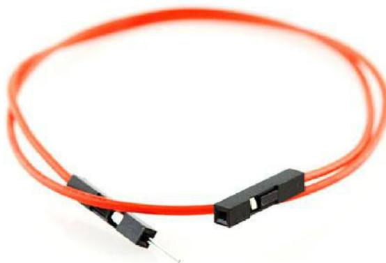
**Gambar 2.10** Kabel *Jumper Male to Female*
