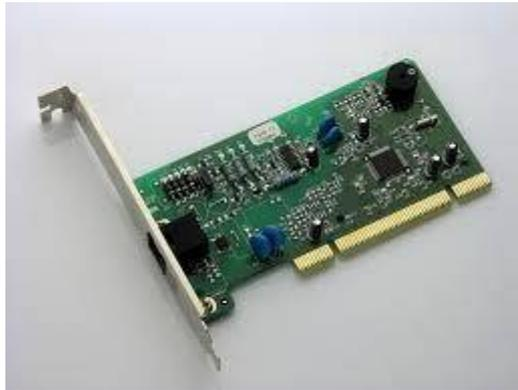
**Gambar 2.12** Modem 56k , Model Internal
