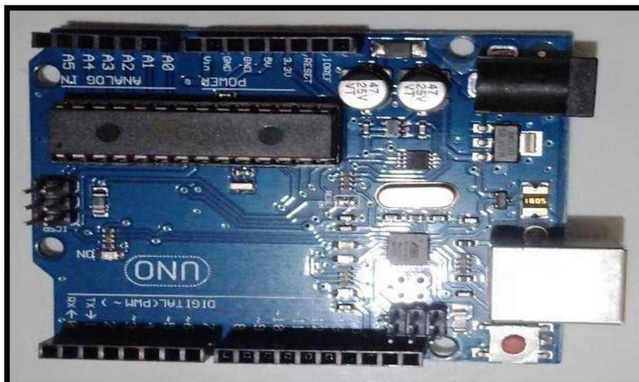
**Gambar 2.4** Board Arduino Uno
