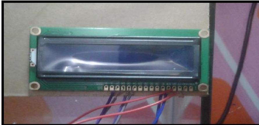
**Gambar 3.16** LCD 2X16
