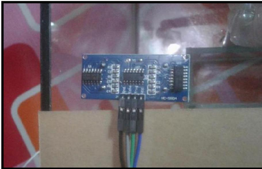
**Gambar 3.14** Sensor ultrasonik
