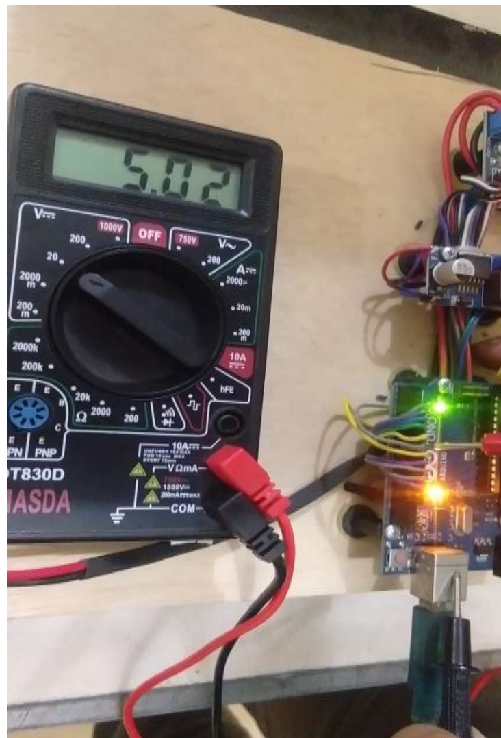
Gambar 4.6 Tegangan photo interrupter kanan terhalang
