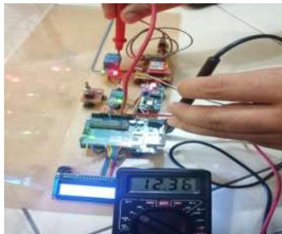
Gambar 4.10 Tegangan *Output Relay* Ke Pompa Air Saat *ON*
