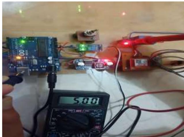
Gambar 4.9 Tegangan *Output* Arduino ke *Relay* Saat *Off*
