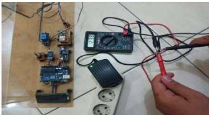
Gambar 4.1 Pengujian Tegangan Output Power Supply
