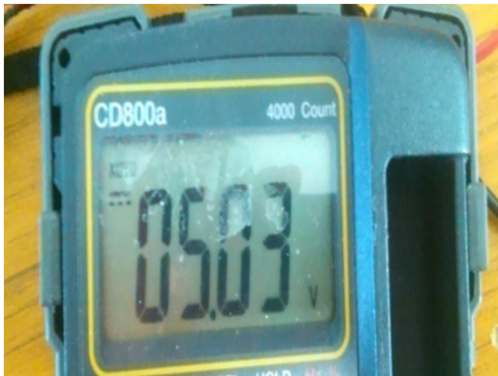
Gambar 4.7 Tegangan Output Ic Regulator 7805.
