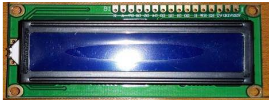
Gambar 2. 9LCD (Liquid Crystal Display) 16x2
