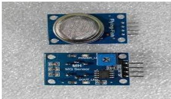
**Gambar 2.9 Sensor Gas MQ-2**
