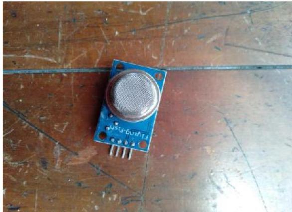
**Gambar 2.7 Sensor Gas MQ-4**
