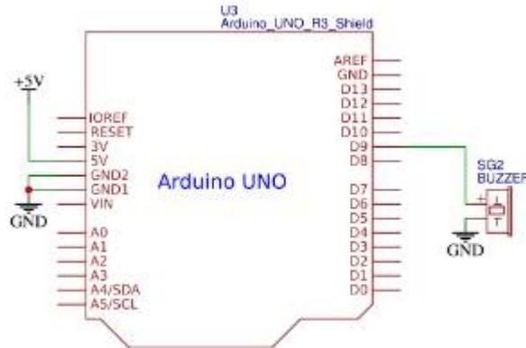
**Gambar 3.4 Skema Rangkaian Arduino Uno Dengan Buzzer**
