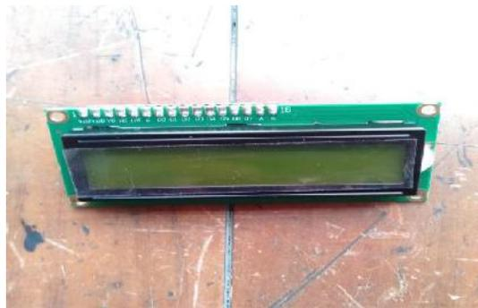
**Gambar 2.10 LCD(Liquid Crystal Display) 16x2**
