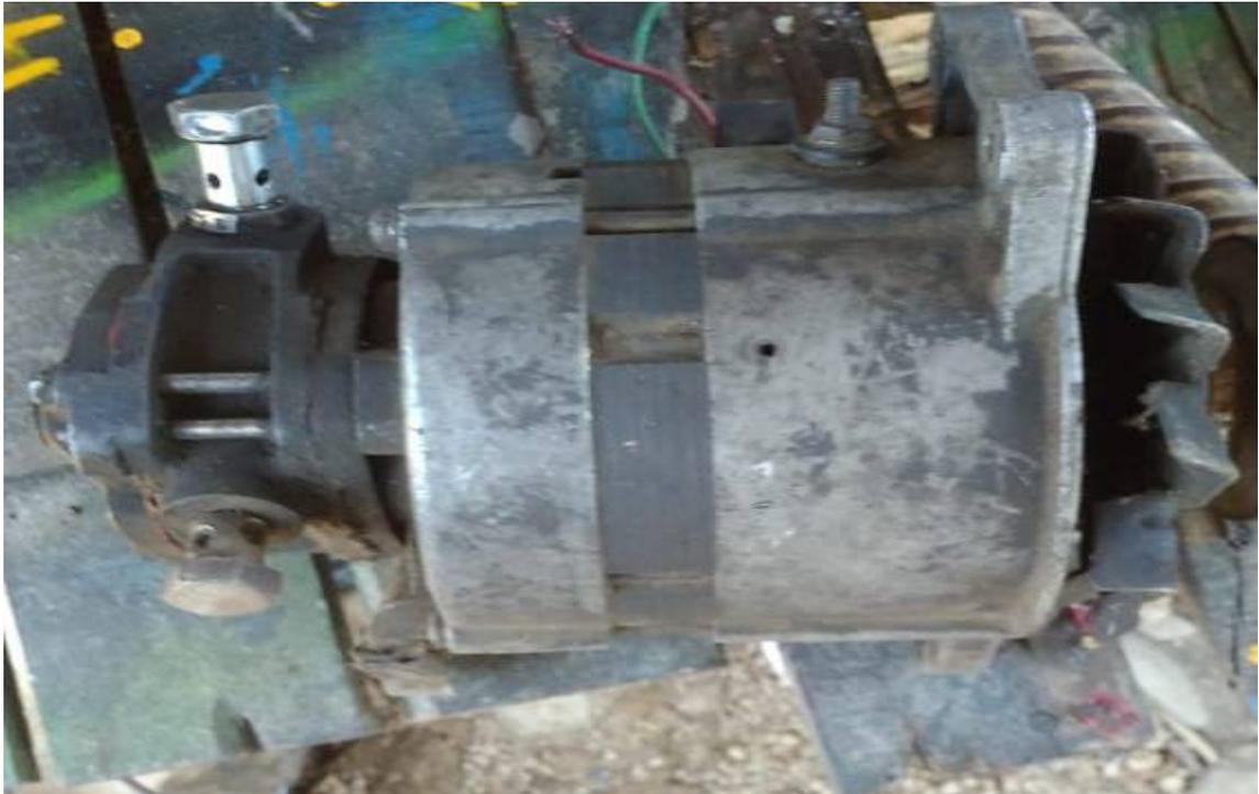
**Gambar 2.1 Alternator DC mobil 12 volt**
