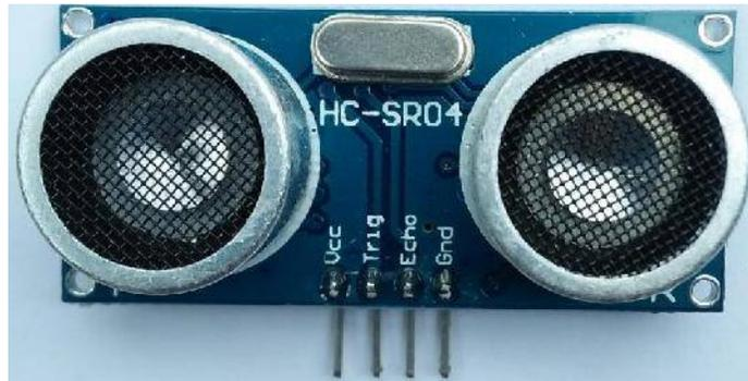
**Gambar 2.6 Sensor Ultrasonik HC SR-04**
