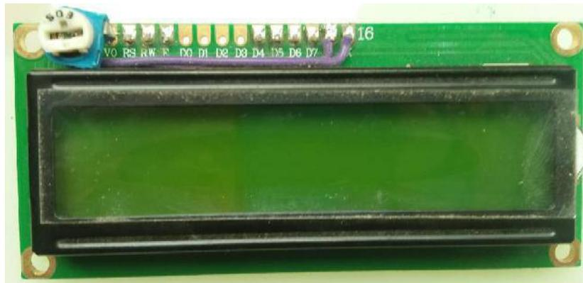
**Gambar 2.8 LCD (*Liquid Crystal Display*) 16x2**
