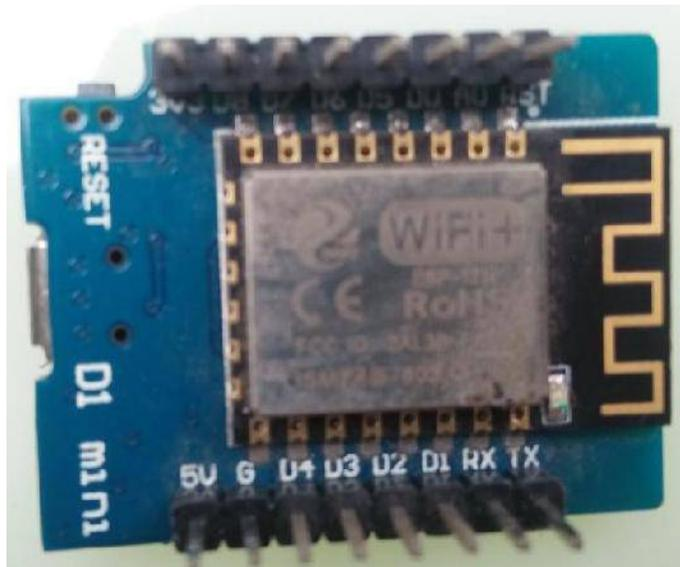
**Gambar 2.7 Modul Wi-fi ESP8266**
