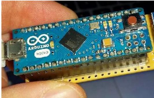
**Gambar 2.10 Arduino Micro**
