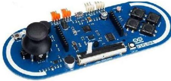
**Gambar 2.12 Arduino Esplora**
