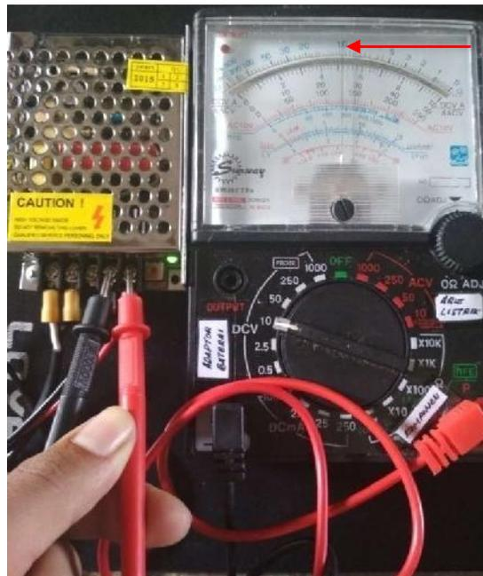
**Gambar 4.1 Pengukuran Output Power Supply**
