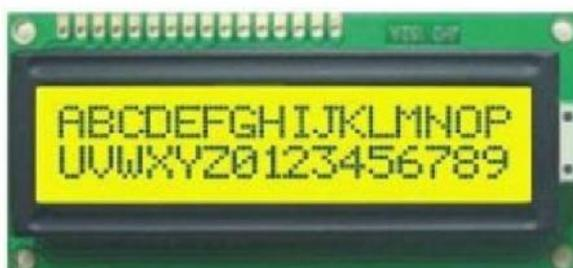
**Gambar 2.10 Modul LCD 16 x 2**
