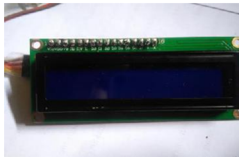
Gambar 4.6 LCD ( Liquid Crystal Display )
