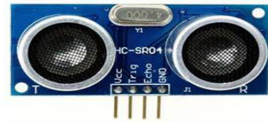
Gambar 2.9 Sensor Ultrasonik HCSR04
