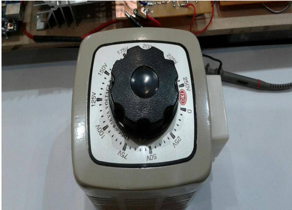
Gambar 4.4 Slide Regulator Transformer 0 – 250 V.
