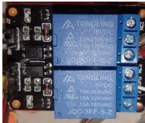
**Gambar 2.2 Relay 2 Channel**
