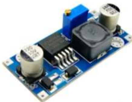
Gambar 2.7 Modul Step Down LM2596 (Sumber : Itead.c, 2017)
