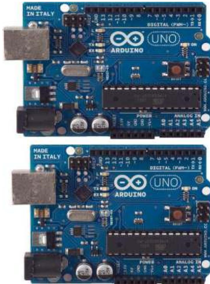
**Gambar 2.1** Board Arduino Uno
