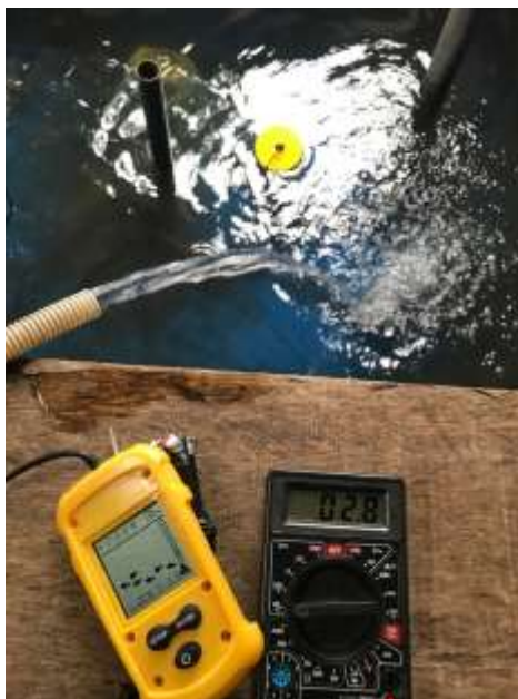
Gambar 4.2 Pengujian Echo Sounder
