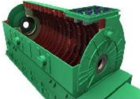
**Gambar 2.1: Stator Frame**
