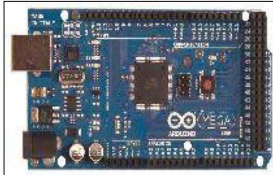
**Gambar 2.8 Arduino Mega 2560**
