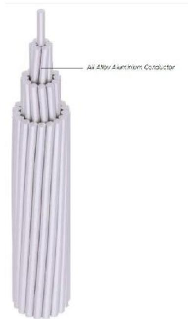
**Gambar 2.14 Kawat Penghantar AAAC (*All Aluminium Alloy Conductor*)**
