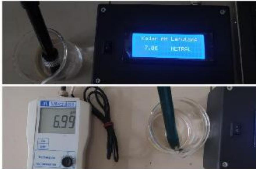
**Gambar 4.11** Proses pengukuran larutan pH *buffer* 7
