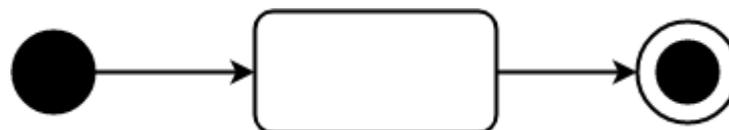
Gambar 2.4 Simbol State Machine Diagram
