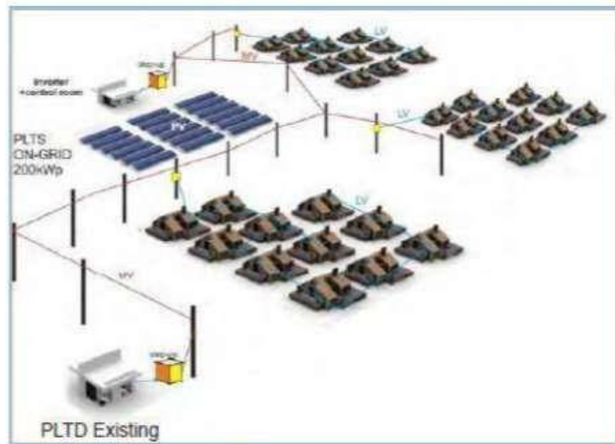
Gambar 2.4 Skema hybrid photovoltaic power system Roihan Abdullah,dkk 2018
