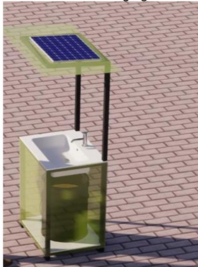
**Figure 4.** Solar Energy-Based Automatic Sink Design
